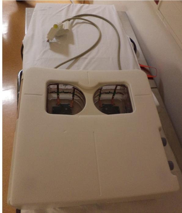
Figure 1.5: Four-channel double-tuned  $^{31}\text{P}/^1\text{H}$  breast coil (Stark Contrast, MRI Coils Research, Erlangen, Germany).
